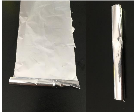
Figure 29 – The whistle was wrapped in aluminium foil to simulate a tube for airflow.
