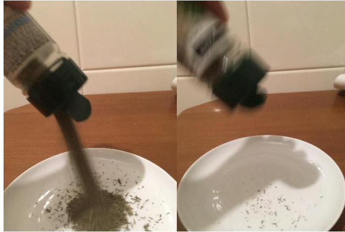
Figure 20 – Two images taken by the author. On the left the jar dispenses the dried leaves at a rate which is very difficult to control using the larger hole setting and, on the right, – almost no dried leaves are expelled of the container using the small hole setting, even when shaken.
