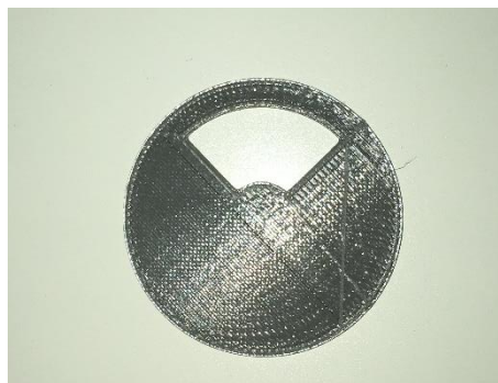
Figure 48 – Top part of the lid with hole for the spices to exit the jar.
