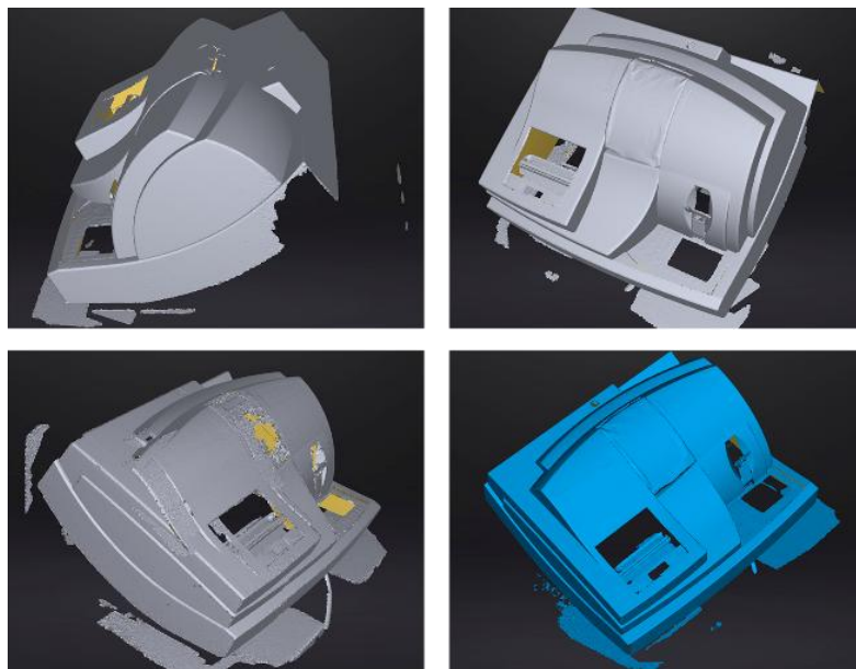
Figure 14 - Initial scan of the equipment viewed from different positions
