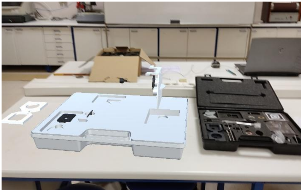
Figure 19 - Model of the suitcase in AR side by side with the real suitcase
