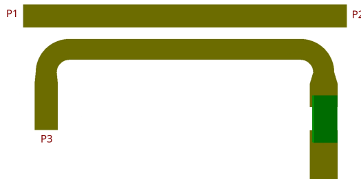
Figure 5.15: Directional coupler EM simulation layout.
