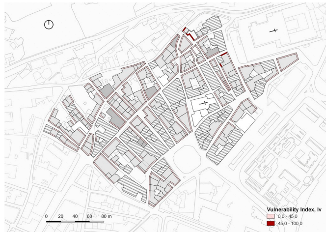
Fig. 20. Façades with I_{vf} over 45, after retrofitting.
