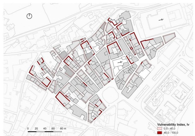
Fig. 10. Identification of the façade walls with I_{vf} values over 45.
