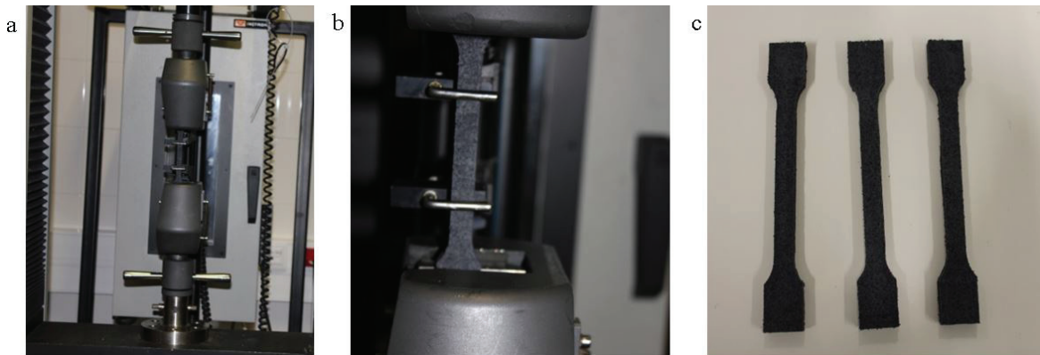
Fig.3. (a) tensile machine; (b) tensile test; (c) tensile samples configuration.
