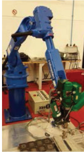
Fig.2. Prototype of the 3D printing equipment developed to produce big green parts.
