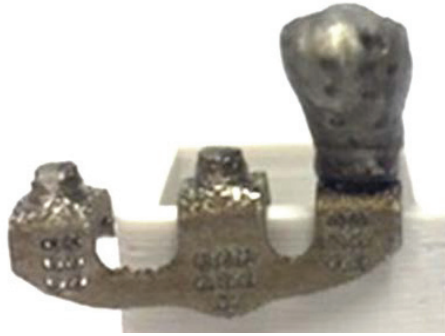
Fig. 4. Multimaterial and personalized physical model of the dental bridge.
