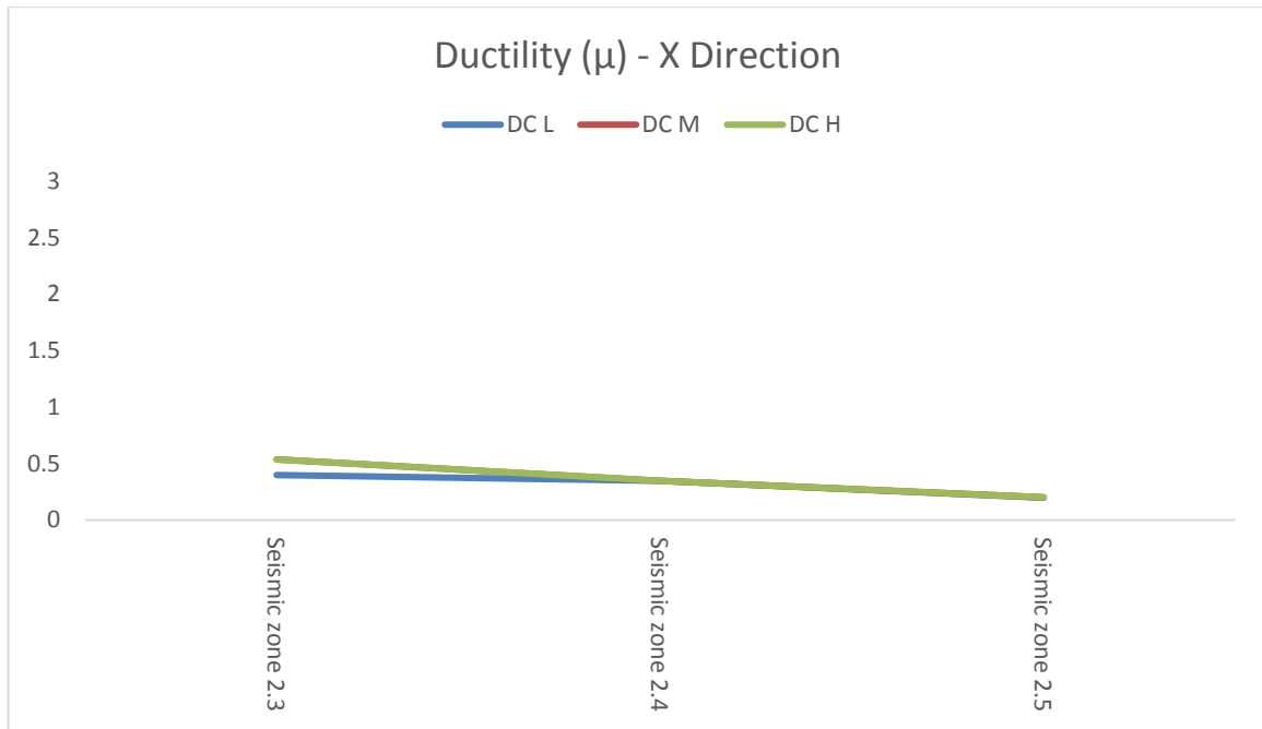
Figure 6.17 Ductility ( \mu ) of seismic actions in X direction, for DC L, DC M and DC H in Seismic zones Type 2
