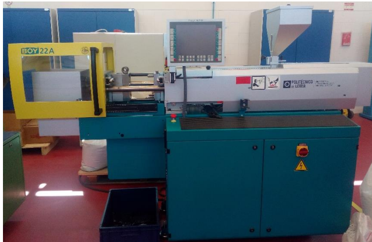
Figure 4- 7 Boy 22A injection machine
