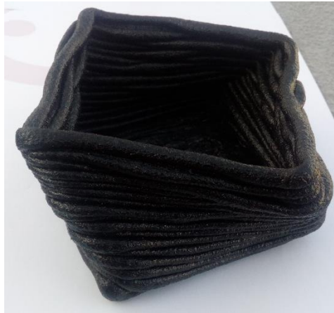
Figure 7- 3 Final result of Additive Manufacturing
