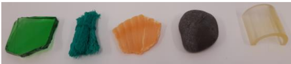
Figure 8 - Examples of the five substrates utilized during the experiment (glass, fishing net, shell, rock, and plastic).
