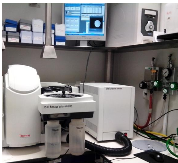
Figure 2.3: Atomic absorption spectrometry with graphite furnace atomization (GFAAS) equipment used on the metal determination.
