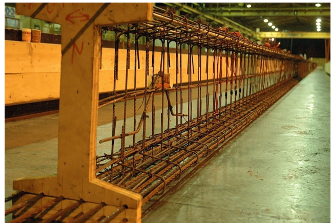
FIGURE 1 Cross-section of the I-girder specimens
