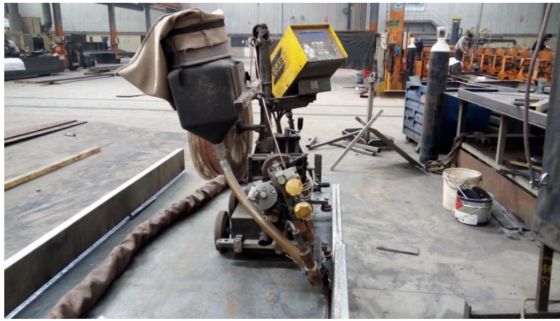
Figure 55: Submerged Arc welding process (Elctrofer Group, 2017)
