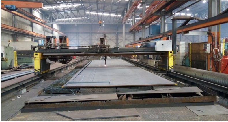
Figure 49: Plasma cut (Elctrofer Group, 2017)
