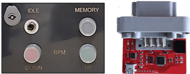
Fig. 6 - (Left) Manual engine speed controller and (Right) Developed electronic speed control module
