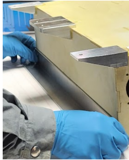
Figure 7.12: L-profile bonding with alignment reference
