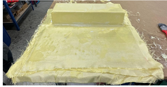
Figure 7.8: Cover lamination in progress
