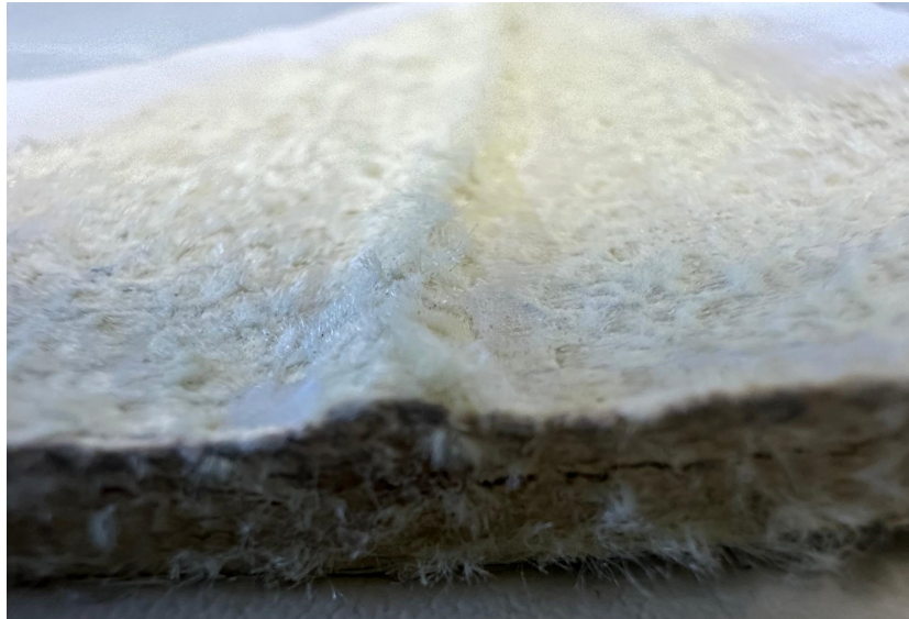
Figure 6.13: Delamination observed in specimen 3 after testing
