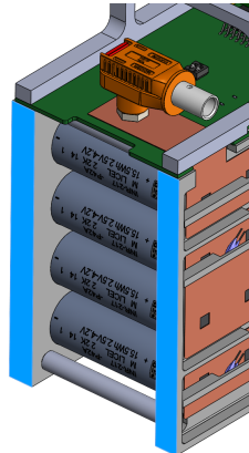
Figure 4.7: Module-to-wall interface - X direction
