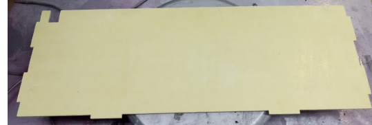
Figure 7.3: Waterjet cut internal wall
