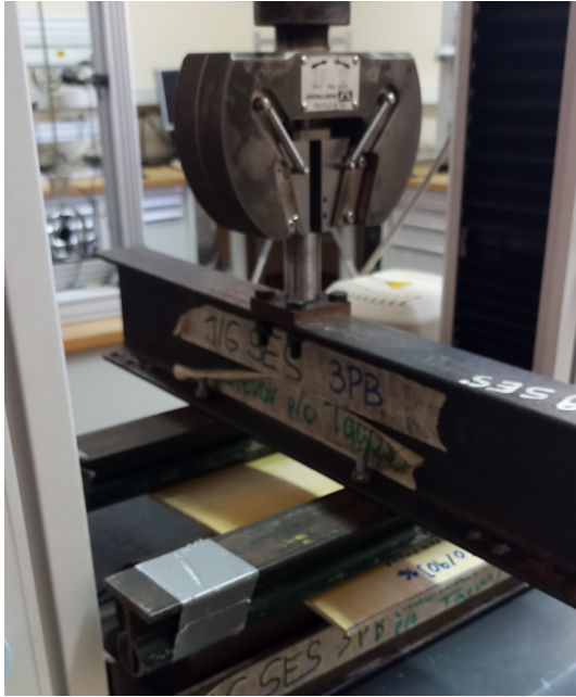
Figure 6.10: Three-point bending experimental setup
