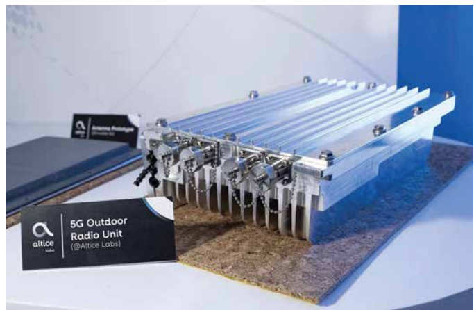
FIGURE 1 – Standard casing solution with embedded antennas
