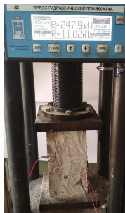
Figure 3.10. – Specimen testing with embedded sensors inside
