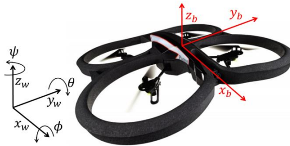
Fig. 6. Global (w) and Local (b) Coordinate systems adopted. [12]
