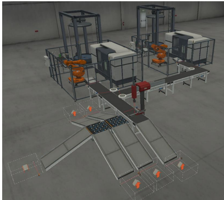
Figure 4.1 – Factory I/O simulation of the automated machining and distribution system
