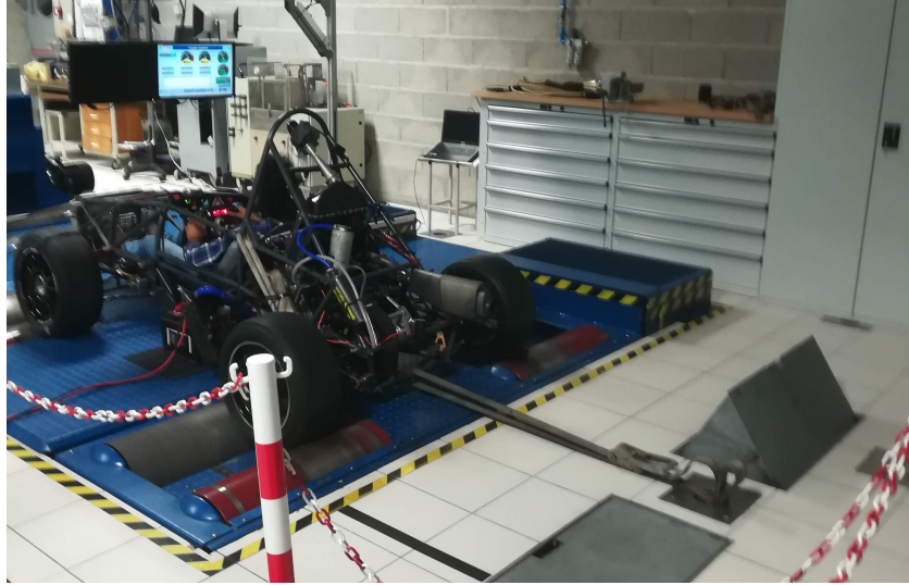
Figure 76: Power dyno trail for measuring engine torque at WOT condition.
