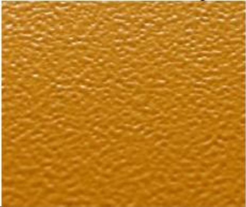
Figure 71: Orange peel (Orange Peel)
