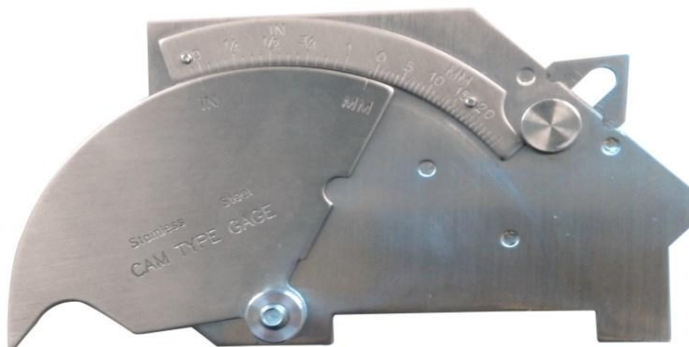
Figure 43: Leg-length measuring cam type gauge (Tools Instruments)
