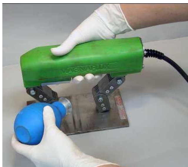
Figure 46: Magnetic particle testing (St. Johns group of Institution)
