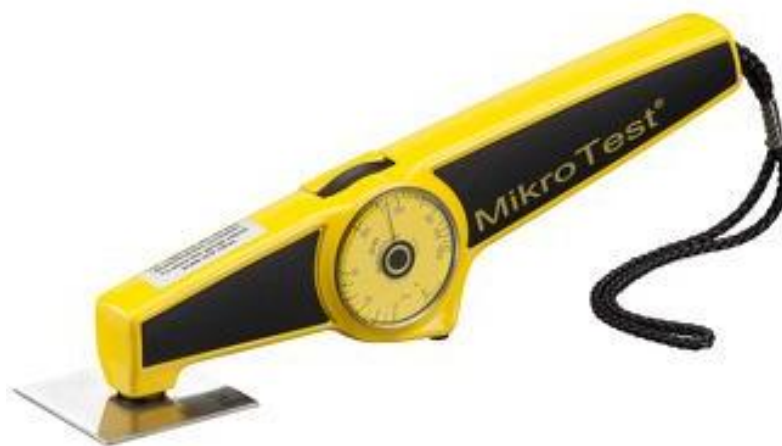
Figure 76: Magnetic pull off instrument for measuring dry film thickness (Magnetic Induction Process)
