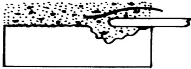
Figure 58: Crevice corrosion (Stainless Steel and Corrosion, 2015)
