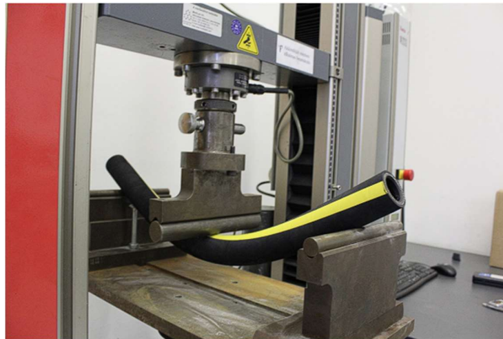
Figura 3.5 – 3 Point Bending Test [29]
