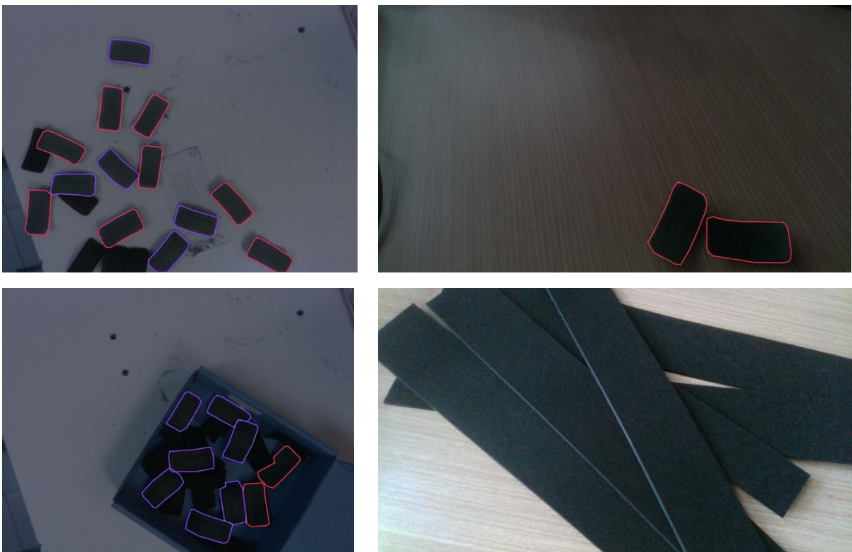
Figure 41: Example of annotated images. Parts labelled as “top” identified in red and “bottom” identified in purple.
