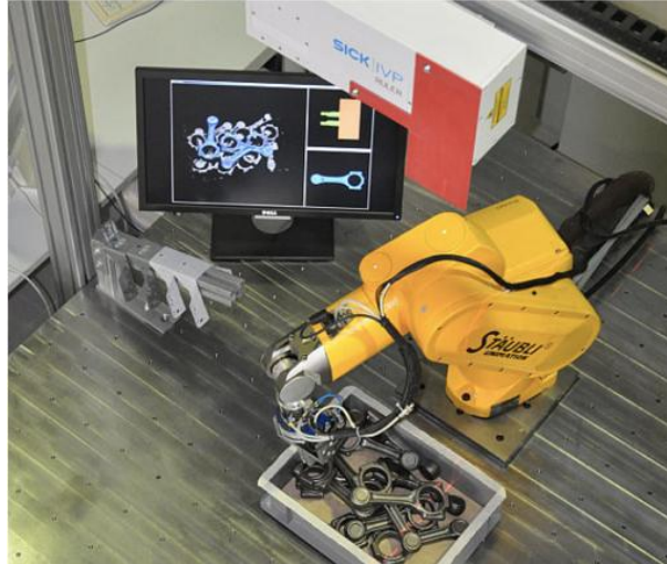
Figure 5: Experimental setup used in Buchholz et al. (2013), consisting of a robotic arm and a laser line scanner.
