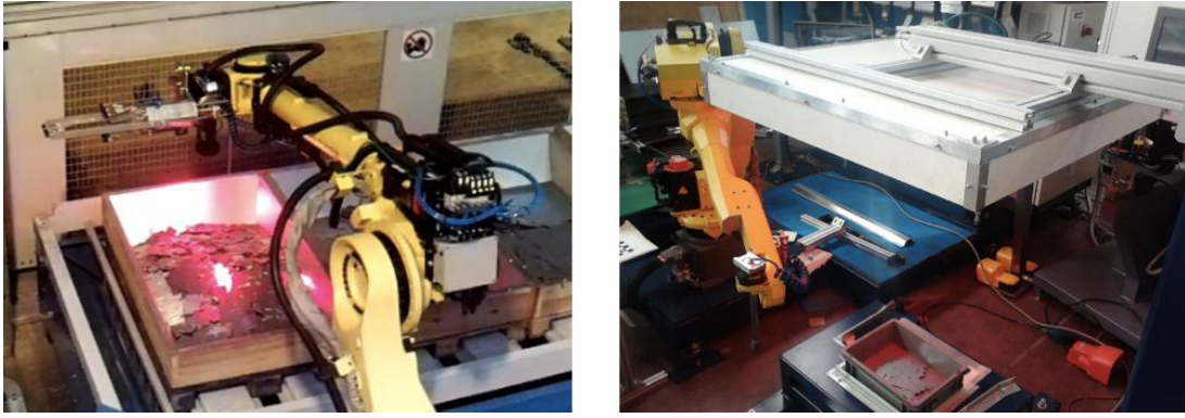
Figure 6: Experimental setups from Pretto et al. (2013). On the left, camera mounted on the robot and on the right, stationary camera.
