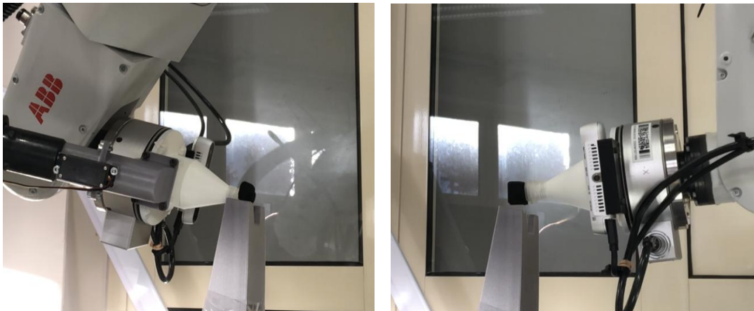
Figure 40: Robot placing the parts in the buffer, according to the side from which the robot picked the part.
