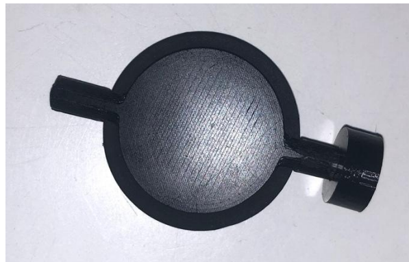
Figure 36: Disc with rubber washer and connector to the servo motor.
