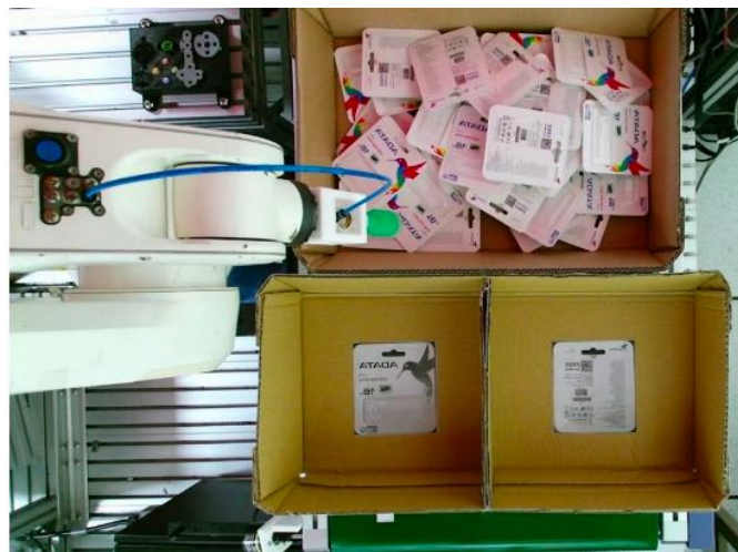
Figure 11: Test setup used in Le & Lin (2019), the robot separates the parts by the side that is facing up in the bins on the bottom part of the image.
