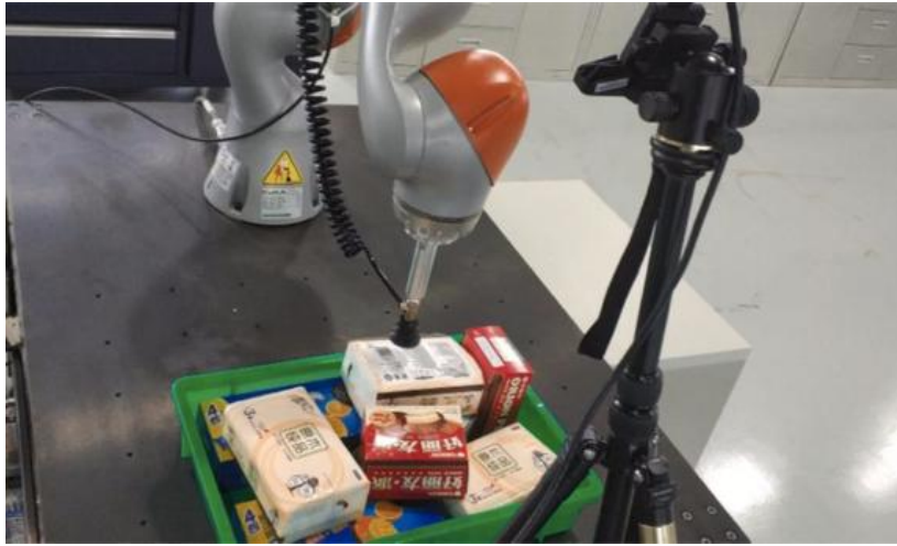
Figure 13: Experimental setup consisting of a robotic manipulator and a vacuum gripper (Zhuang et al., 2021).
