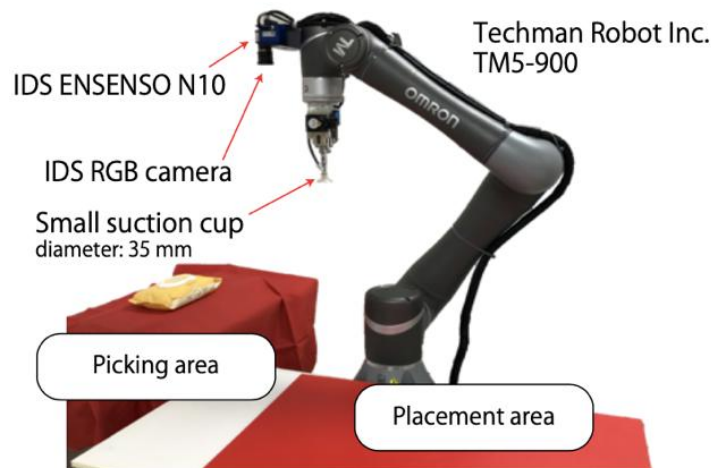
Figure 12: Test setup proposed in Araki et al. (2020), consisting of a robotic arm, a RGB camera, a depth sensor and a vacuum gripper.
