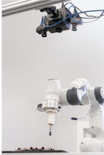
Figure 14: Setup consisting of a robot, a RGBD camera and a vacuum gripper (X. Li et al., 2022).
