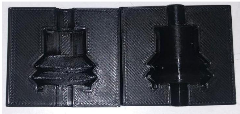
Figure 31: Mould to produce the personalized suction cup.
