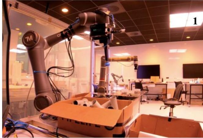
Figure 15: Test configuration from G. Li et al. (2023), consisting of a robot, 3D vision system and a vacuum gripper.
