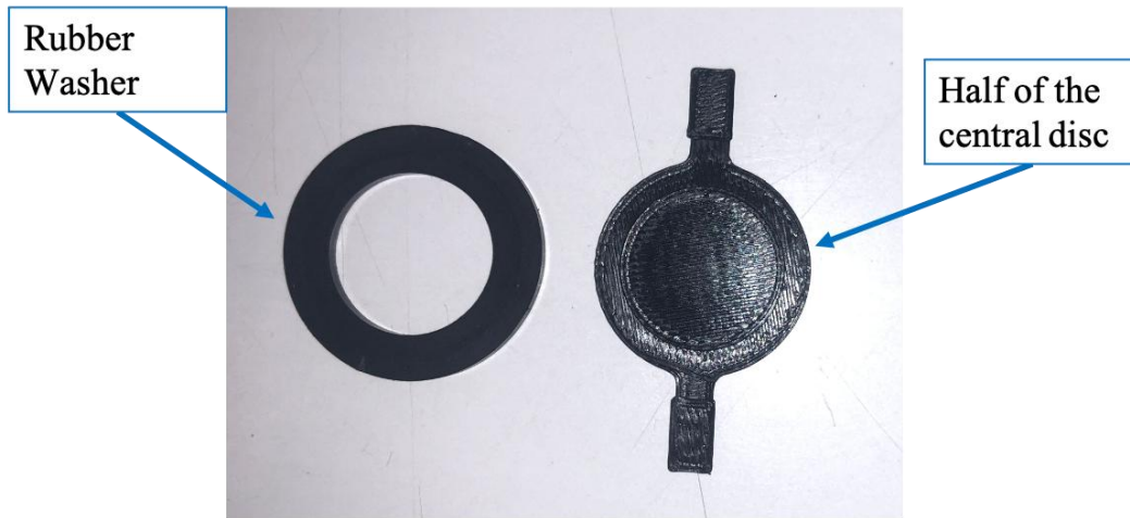
Figure 35: Components of the second version of the butterfly valve.
