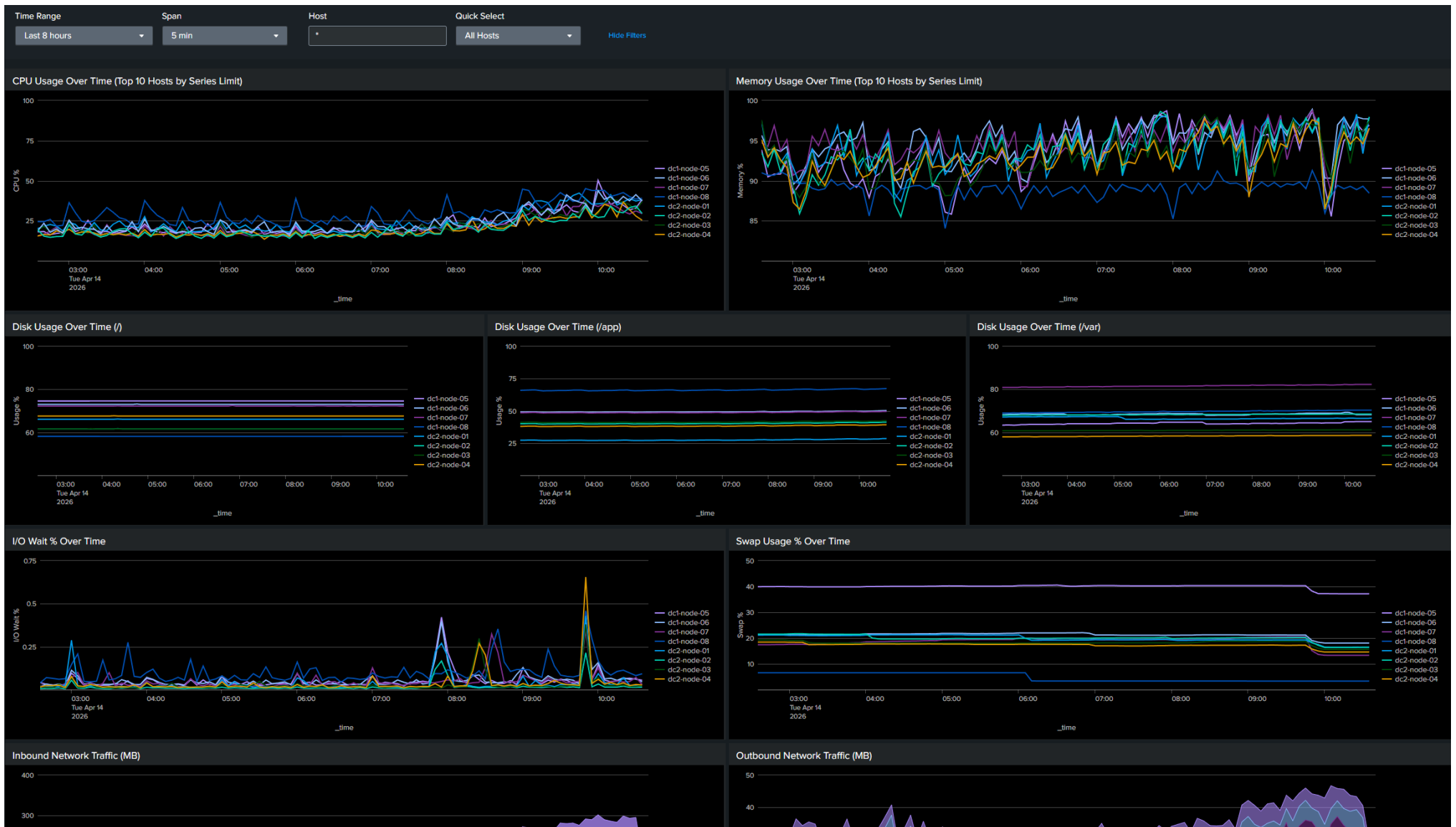
Figure B.3: Performance tab with time-series CPU, memory, disk, I/O wait, and swap monitoring
