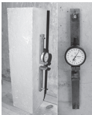
Fig. 2 Shrinkage measurement. Fig. 3 Evolution of concrete shrinkage strain.
