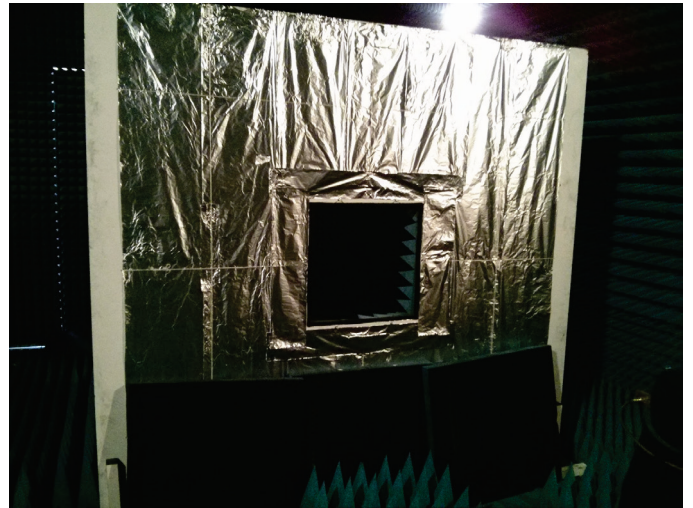
Figure 4. Back view of FSS support structure.
