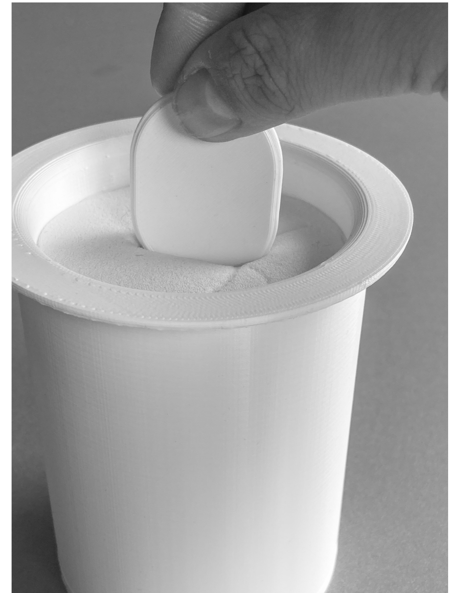
3-D printed model of the initial design of the sensor pre-cleaning and disinfecting unit to be used in the HED.
