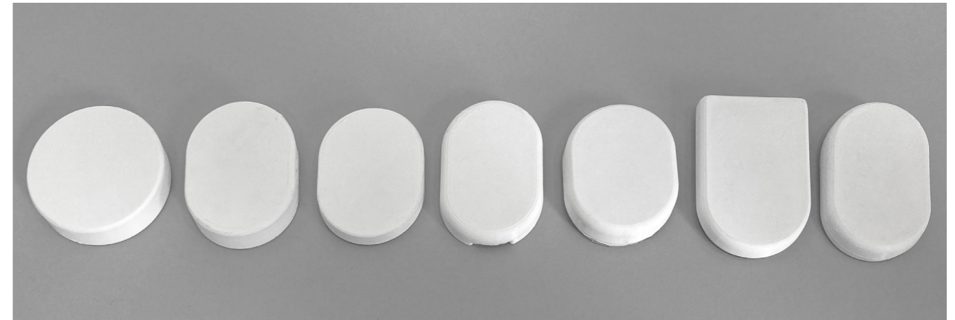
3-D printed models of various sensor capsule shapes and the peel-off section.
