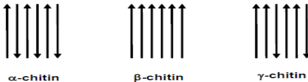
Figure 4 - Arrangement of the polymer chains in the three forms of chitin. Source: Einbu, 2007.
