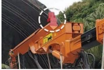
Figure 2.4: The 2-D scanner mounted on the robotic arm used to generate 3-D models (taken from [9]).
