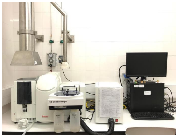
Figure 6: Atomic Absorption Spectrometer (Thermo Scientific™ iCE™ 3500 Atomic Absorption spectrometer, Thermo Unicam, Portugal).
