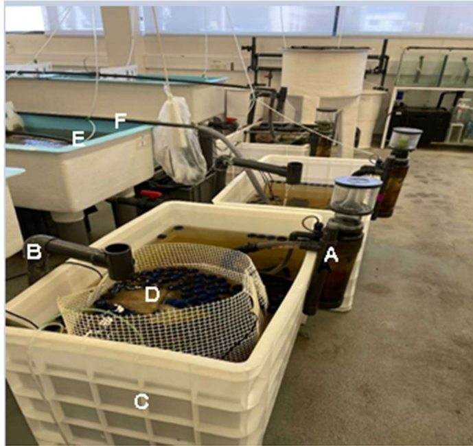
Figure 5- Sump with mechanical and biological filtration from each RAS system where: A- skimmer, B- water exit tube, C- water compartment, D-sponges and bio-balls, E- aeration stone, F- water entrance tube.
