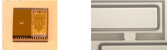
Fig. 1. (a) SAES dice (dimensions: 6 × 6 mm); (b) Detail of the accelerometer beams shape and proof mass edges (bottom view).
