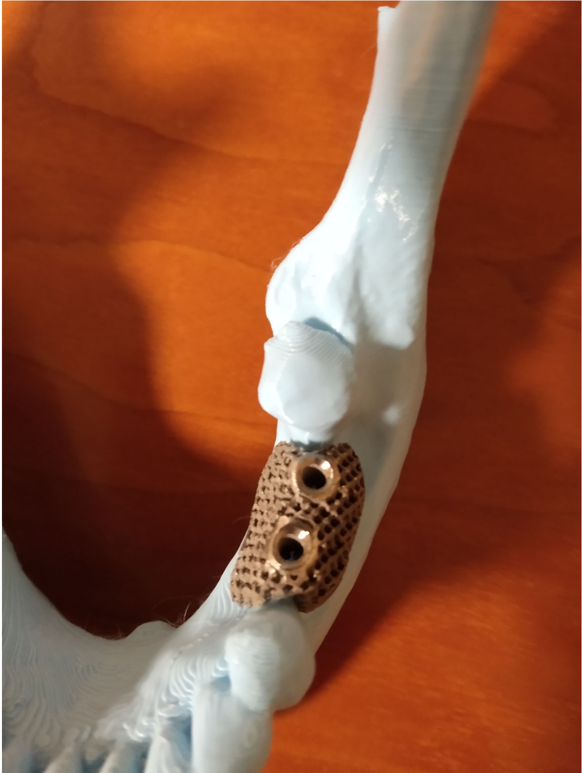
Figure 4.43: DESIGN LINE 3, Titanium EBM printed prototype
