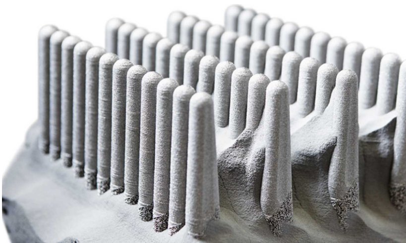
Figure 3.17: EBM Base plate + printed pieces + unsintered powder
