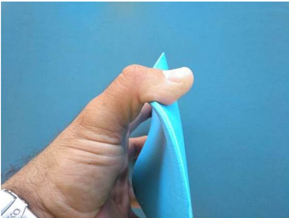
Figure 4.21: TPU flexible printed prototype
