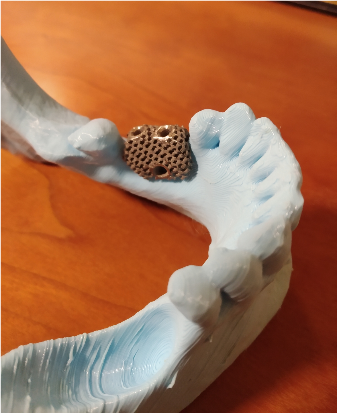
Figure 4.45: DESIGN LINE 3, Titanium EBM printed prototype
