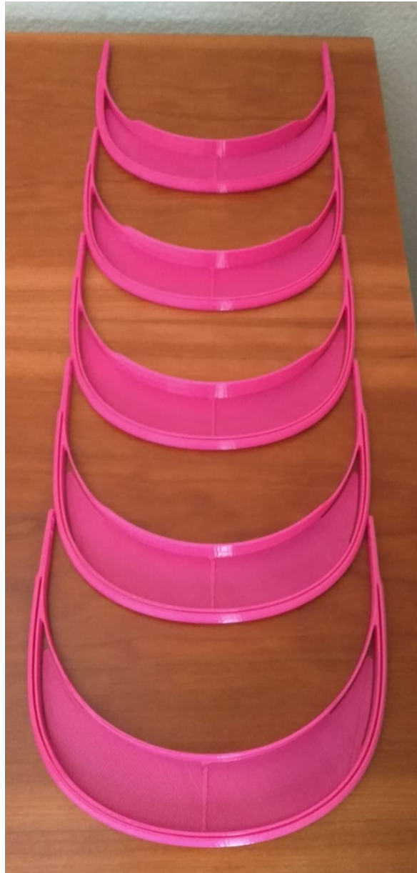
Figure 5.6: FDM printed Face shield structure
