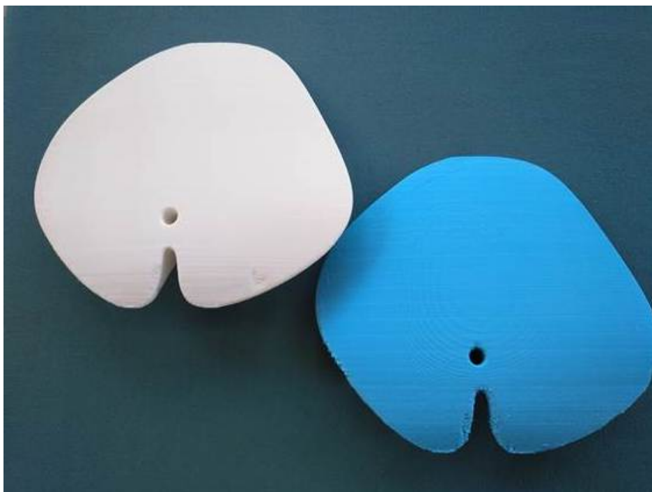
Figure 4.18: TPU flexible printed prototype
