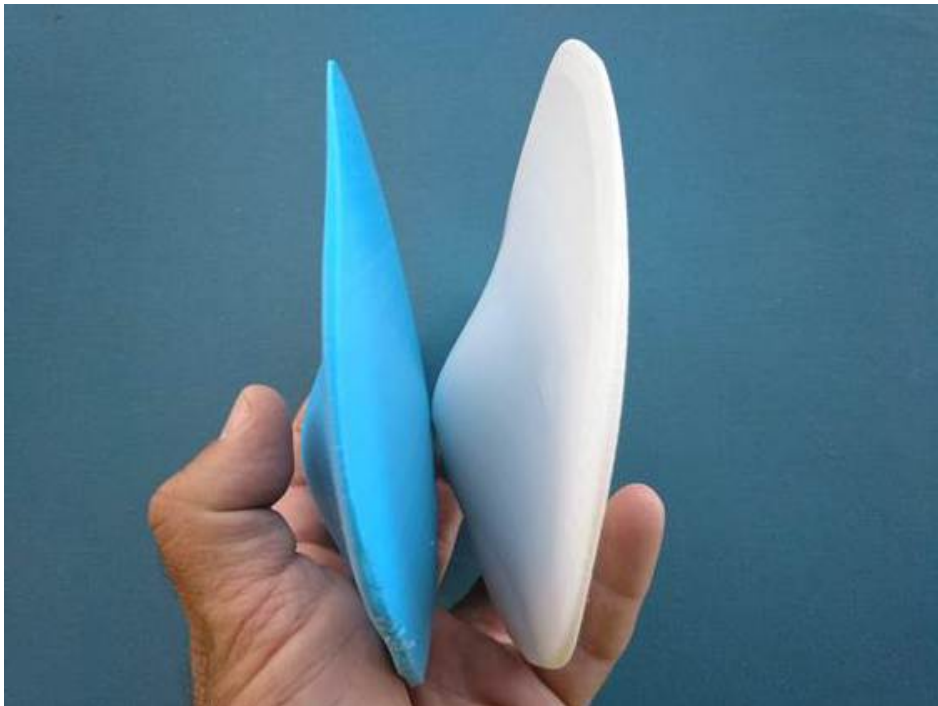
Figure 4.20: TPU flexible printed prototype
