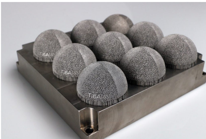
Figure 3.18: EBM Base steel plate
