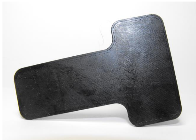
Figure 51 - First layer after 6 hours of material dehumidification.
