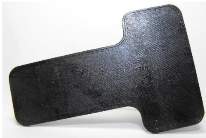
Figure 48 - First layer after 3 hours of material dehumidification.
