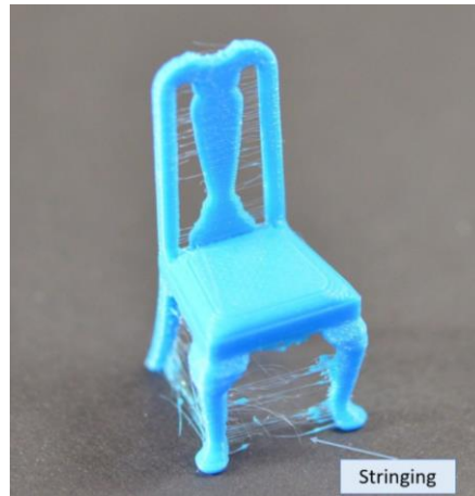
Figure 17 - Printed part with stringing [22].
