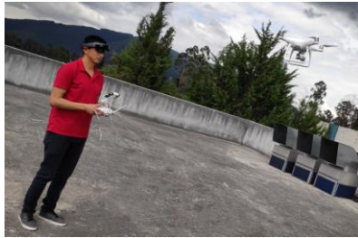
Figure 3. Phantom 4 controlled by HoloLens
