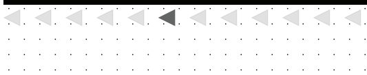
FIGURE 14: Possible signal emitter locations near a wall. Light gray triangles are the possible locations for the placement of signal emitters, while the dark triangle is a placed signal emitter.
