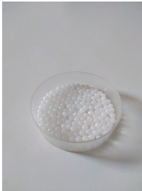
Figure 3.10: Samples of virgin HDPE used for the absorption tests.
