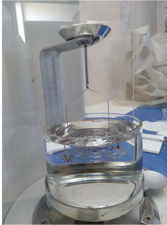
Figure 3.11: Equipment used to determine the mass and impulsion of each sample.
