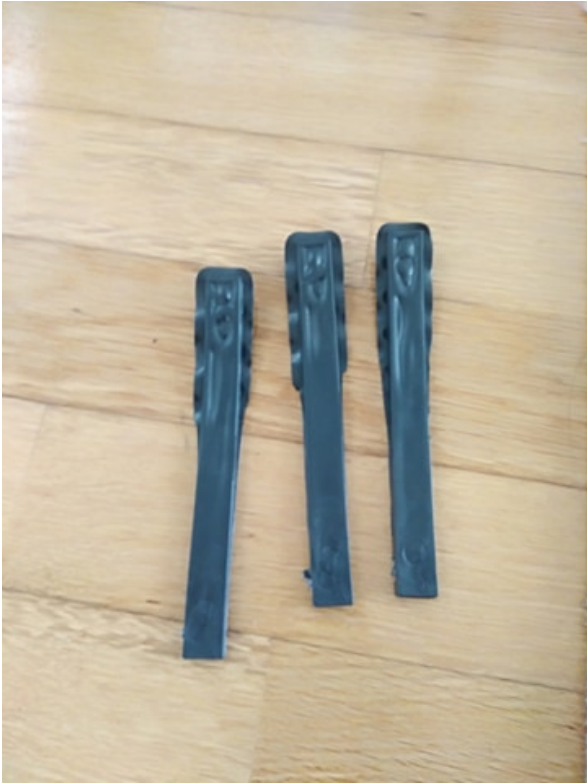
Figure 4.4: Homogeneity obtained on the specimens due to the material's injection difficulties.
