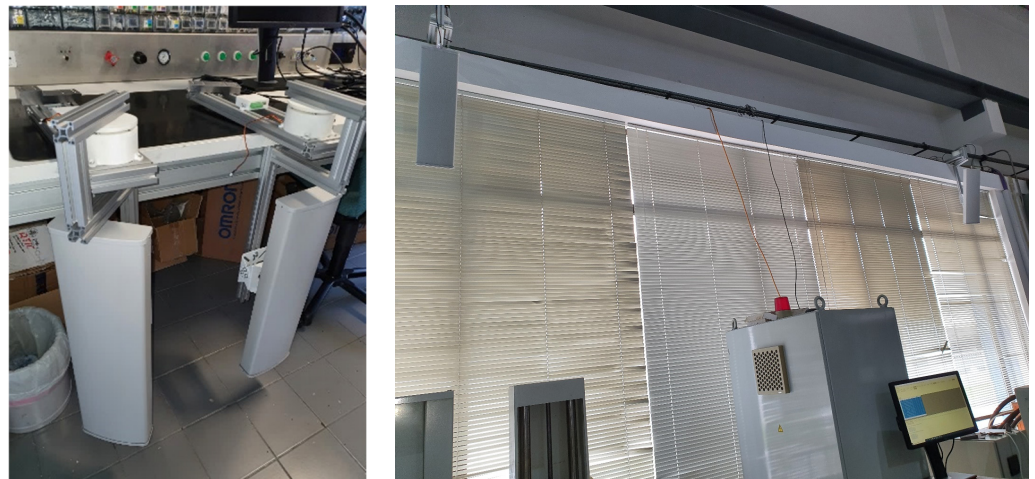
Figure 8. RFID antennas over rotating bases.
