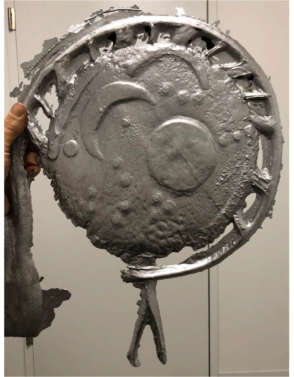
The rough casting is complete with its large sprue, multiple gates, and two V-shaped vents.
