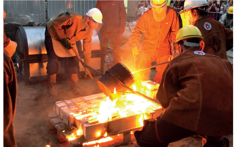
Above: Pure iron is carefully ladled into the awaiting molds, often resulting in dramatic fireworks.
