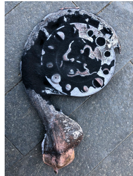
Carbonized sand is first removed by brushing and later by sand blasting.
