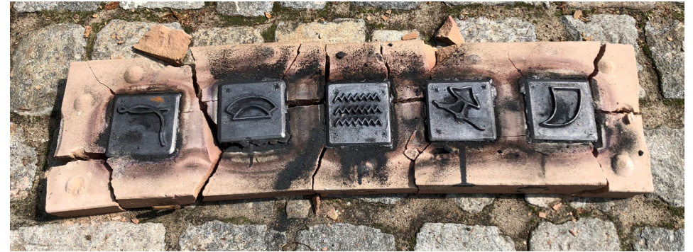
After the two parts of the mold have been separated, a hammer was used to break apart the rock hard mold.
