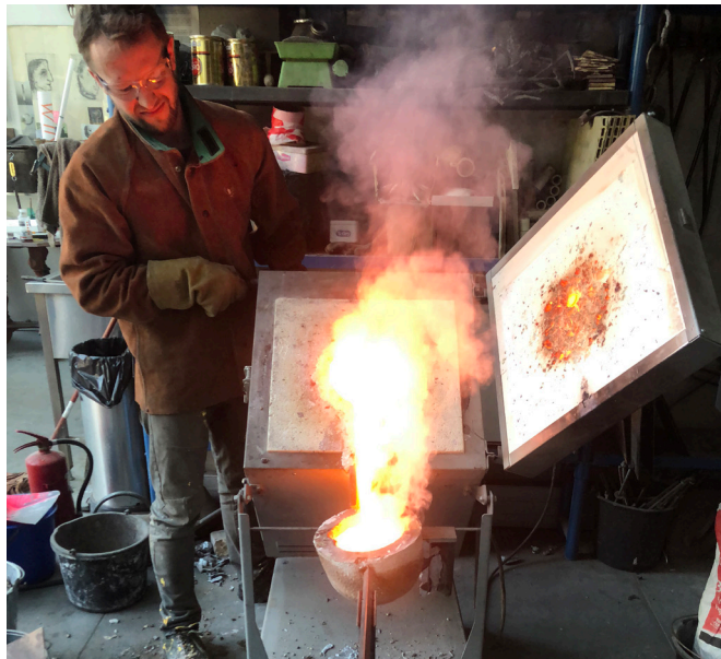
Once impurities have been removed from the melted charge, and adequate temperatures have been achieved, the liquid alloy is carefully poured, or tapped, into the crucible.
