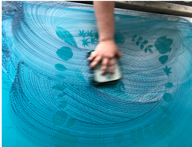
Right: The plate is exposed on a light table and developed with an alkaline solution, and rinsed with water creating a positive hydrophobic image.
