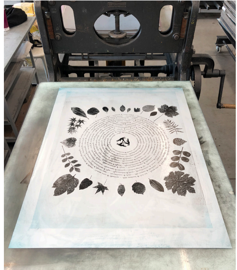
To print, paper is placed on the stone, followed by a sheet of newsprint and blotter paper. Then a sheet of smooth resistant material known as a tympan is laid on top. The tympan can withstand the enormous pressure without deforming. The bed is raised into position and small amount of grease is evenly distributed along the scraping bar. It is all fairly simple.
