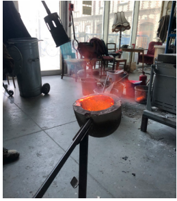
A ladle, known as a crucible is used to transfer molten metal from the furnace to the flasks. Preheating is essential for reducing thermal stress on the crucible.
