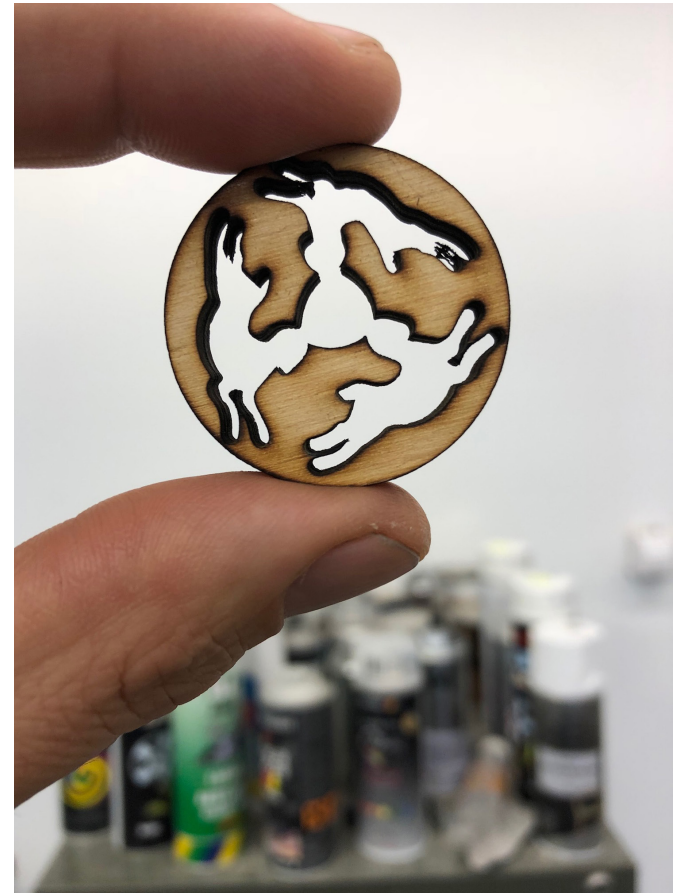
Above right: A CNC laser cutter was used to create a series of circular templates on 3mm plywood.
