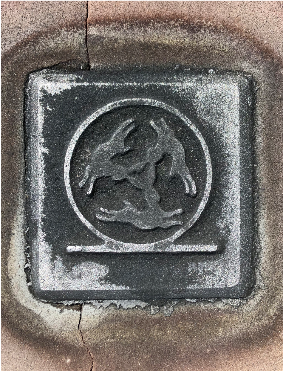
Still embedded in the mold, the resulting designs are crisp and detailed indicating a very successful pour.
