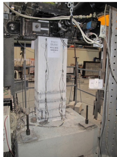
Fig. 1. a) RC column specimen dimensions and reinforcement detailing; b) General view of the test setup at LESE Laboratory.
