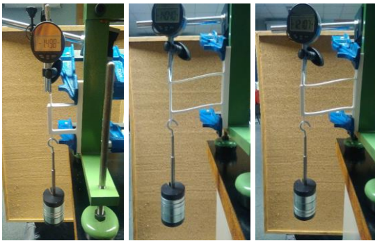
Figure 5. Displacement tests for 3D-printed single-bay frames using ABS.
