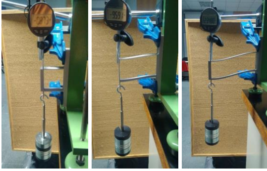
Figure 4. Displacement tests for 3D-printed single-bay frames using PLA.
