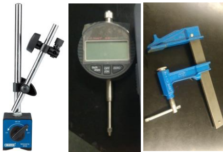
Figure 7. Magnetic stand (left), digital indicator probe (center) and clamp (right) used in the analysis of plane frames.
