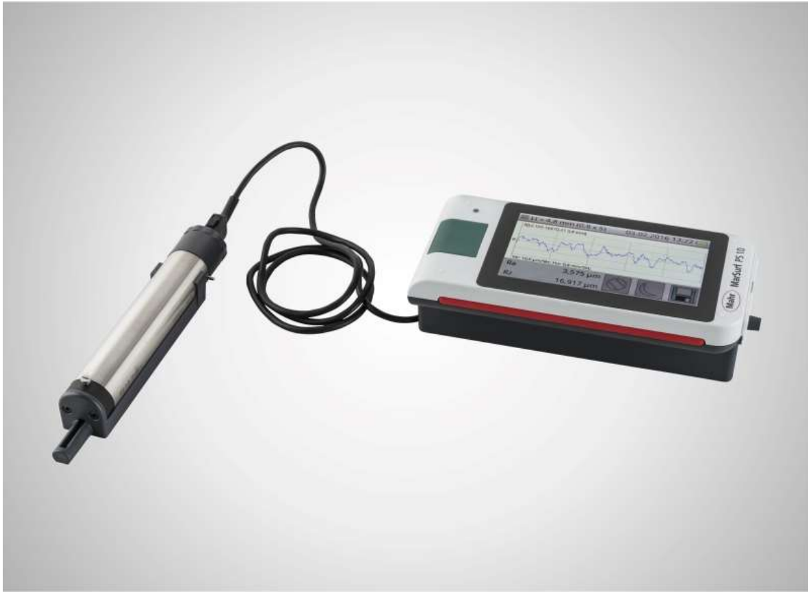
Figure 51 Perthometer with Stylus needle [23]
