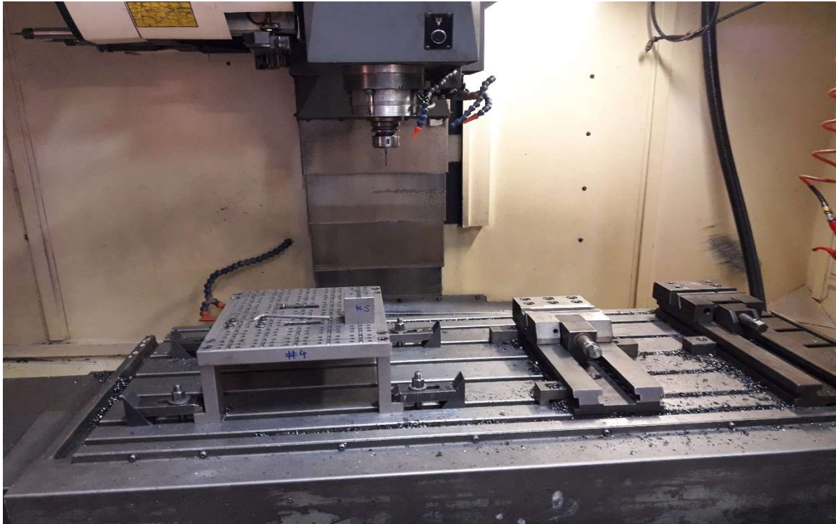
Figure 21 Working surface of Hartford Omnis
