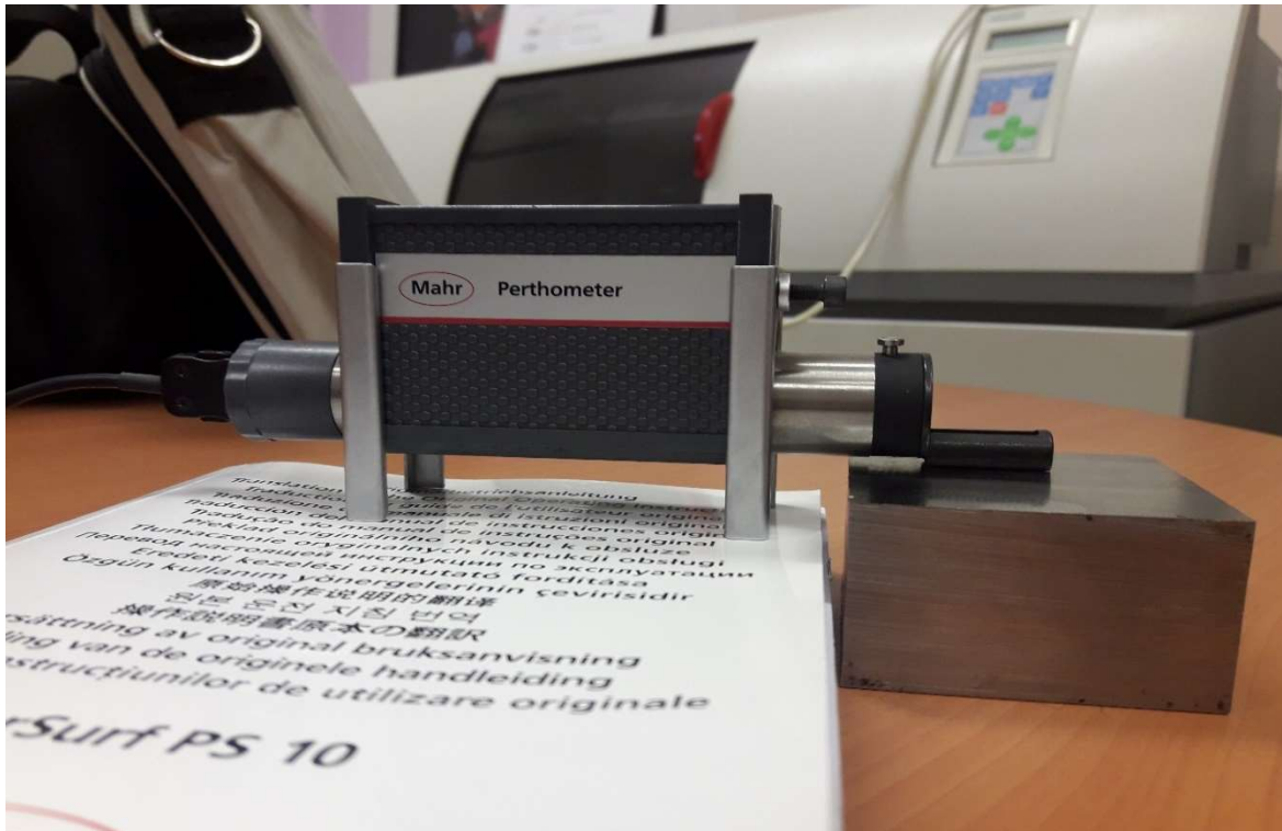
Figure 52 Roughness test on steel 1.2316
