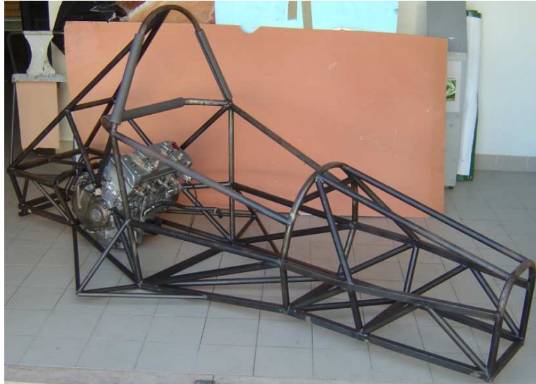
Figura 6 – Chassis tubular do Formula IPLeiria.
