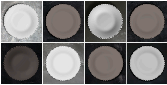
Fig. 5. Domain randomization example of synthetic data in a fixed placement industry environment with CeramicFlow .
