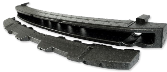
Figura 9 - Para-choques automóvel de Polipropileno Expandido (Engineered Foam Products, s.d.)
