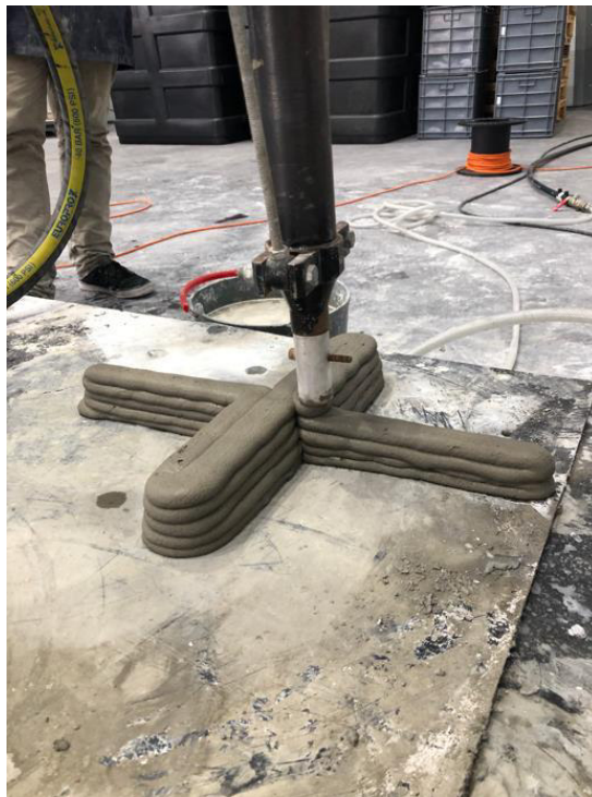
Figure 4.7: Printing test - mix 21
