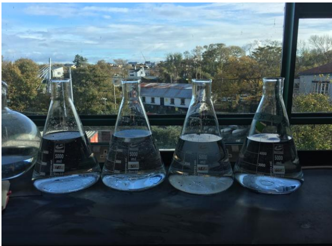
Figure 3.6: The four salinities 16‰, 32‰, 48‰ and 64‰ prepared for the first treatment.
