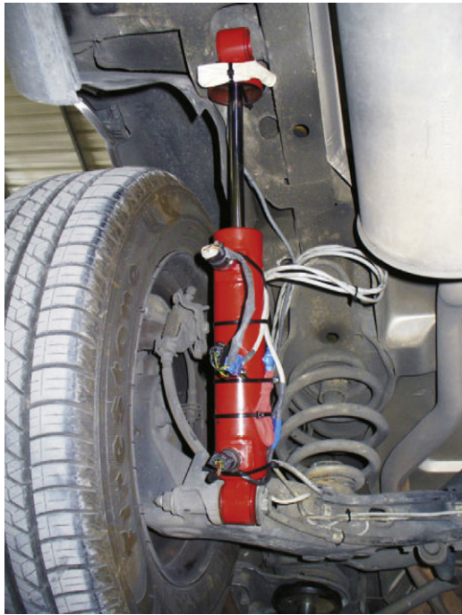
Fig. 9. Instrumented shock absorber installed in a test vehicle.
