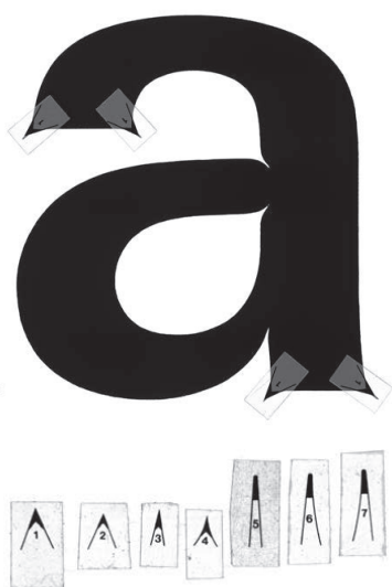
Figure 13. (a) of Universe (1957) as designed for filmsetting (top), and adjustments required for accurate reproduction (bottom), found in (Osterer, 2012, p.104).
