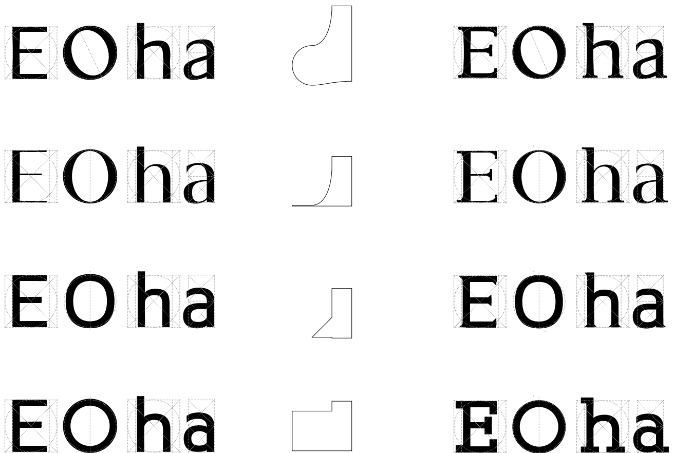
Figure 61. Fixed heartlines with no value for serif width, serif height, and bracketing (left) augmented by master serif outlines (middle), and resulting typographic style (right).
